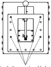
Align bottom seat pad holes with these four hole locations
